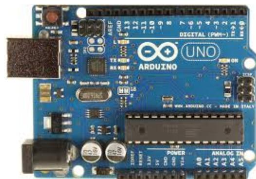
Arduino circuit board
